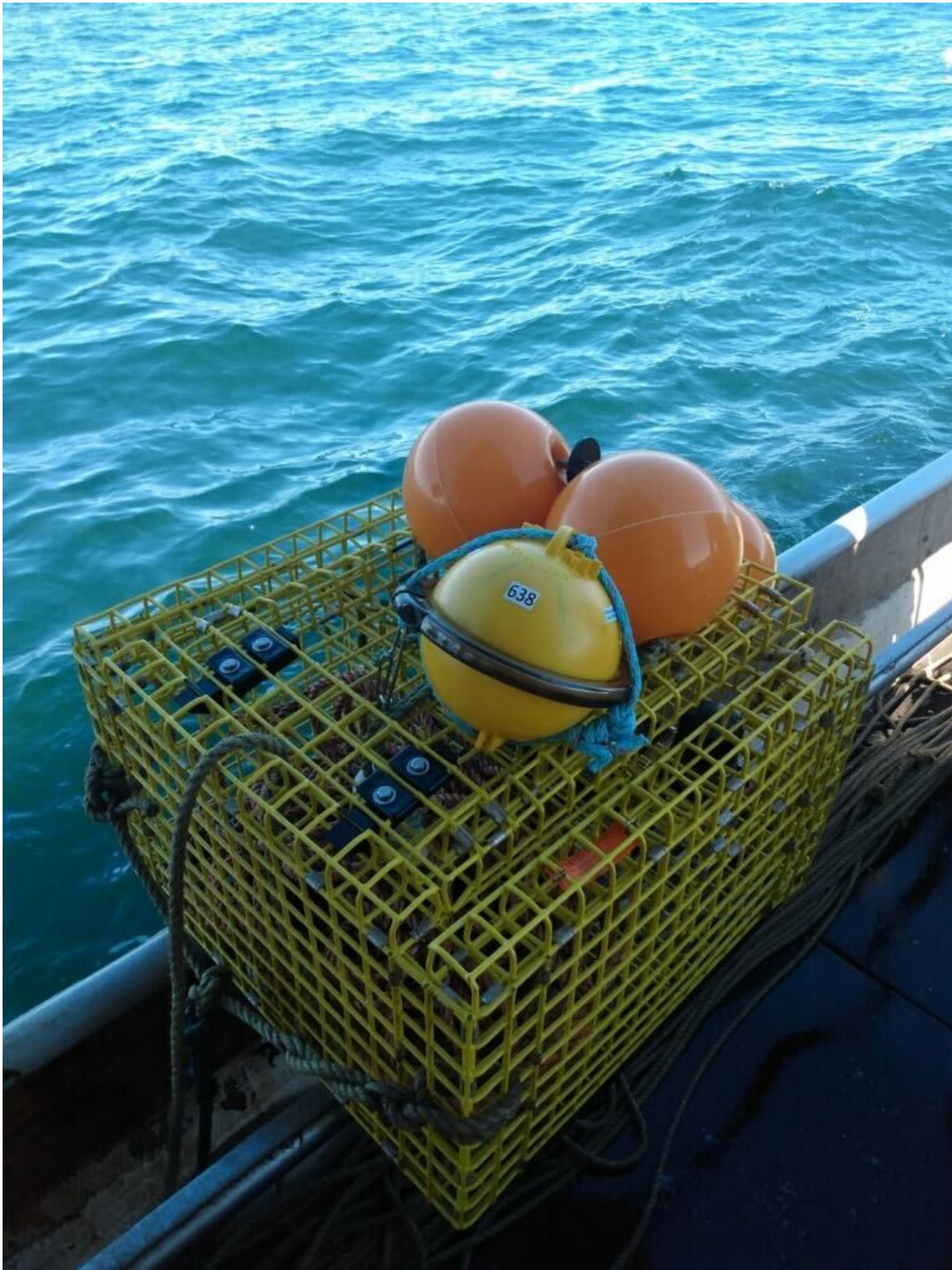
Smart Buoy installed on On-Demand gear during zone closure
