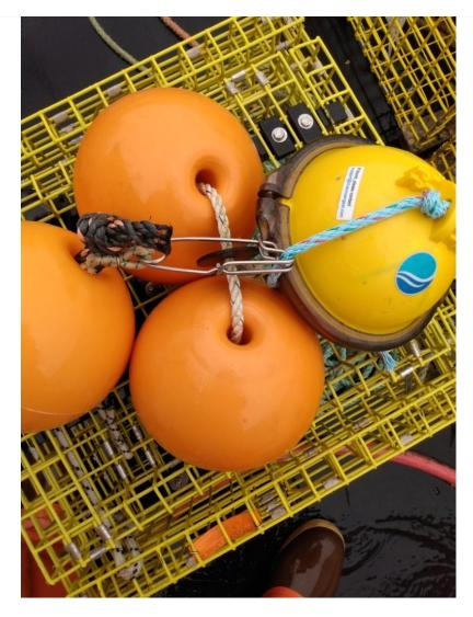
At Blue Ocean Gear, we know that surface gear doesn't always stay on the surface. Our Smart Buoys are depth rated to 300 meters (or 164 fathoms). This allows our sensors to distinguish between an entanglement and other events such as gear conflict.
